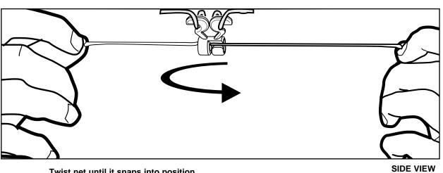
Twist net until it snaps into position. Net must be centered through clip.
